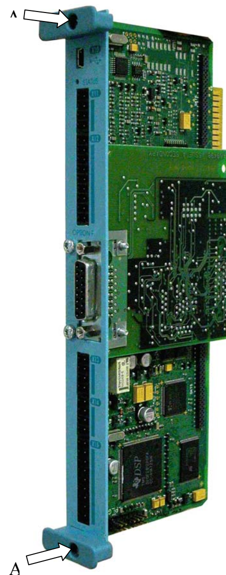
Figure A-1 Control board with an Option Card correctly mounted
